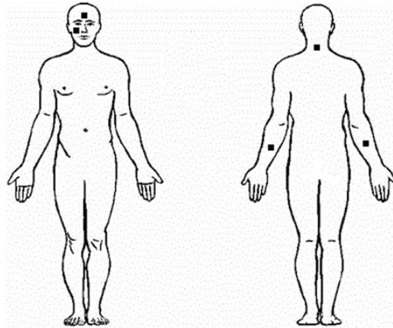
**Figure 1. Dosimeter locations on the workers' bodies.**
